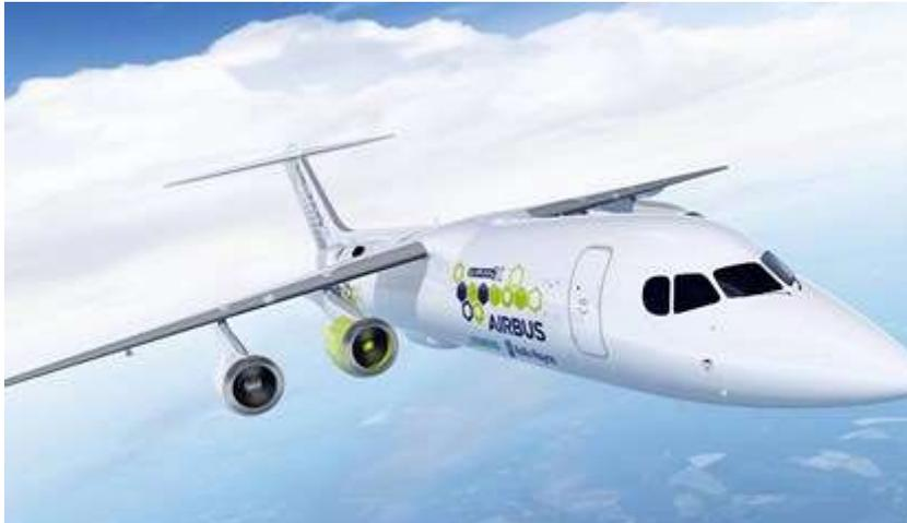
Airbus, Rolls-Royce and Siemens recently announced plans to use a BAe 146 as a hybrid electric aircraft test bed. (Airbus)
