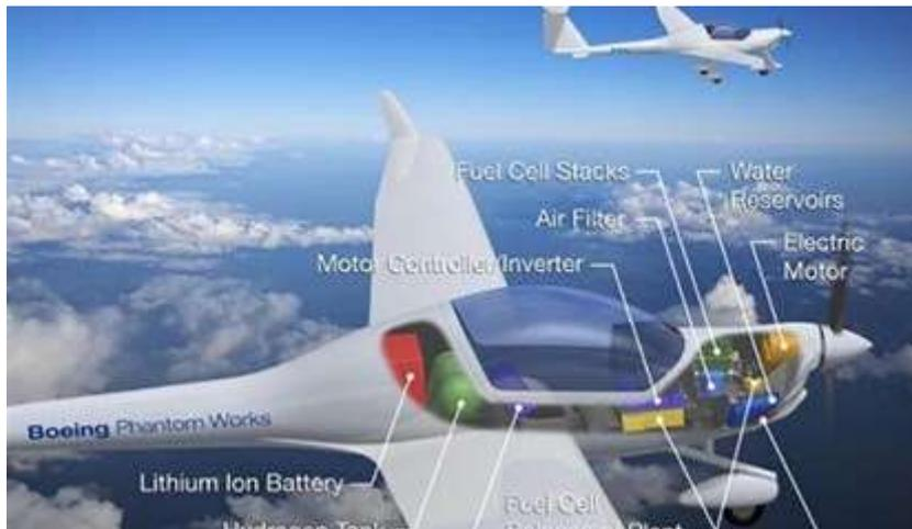
Boeing Phantom Works' electric-powered demonstrator was powered by a hydrogen fuel cell and a lithium ion battery located inside the fuselage. (Boeing)
