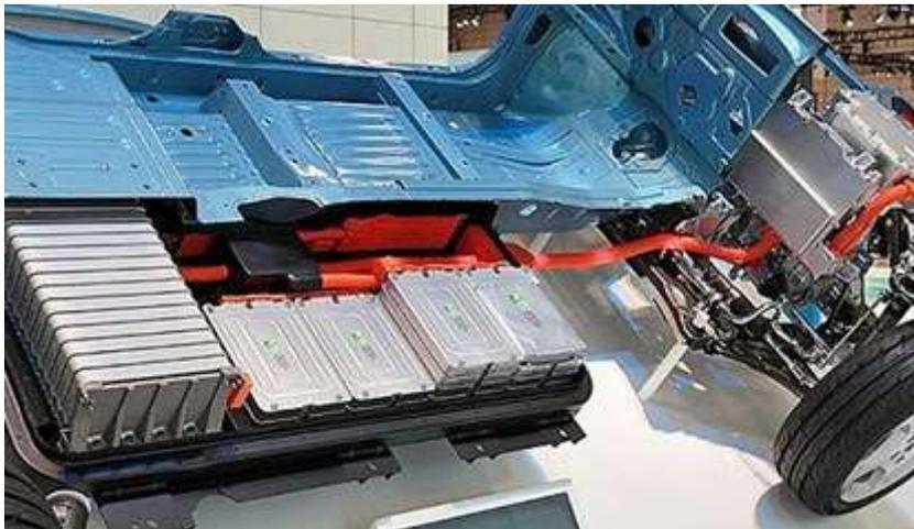
Lithium-ion batteries fitted on a Nissan Leaf electric car. The development of the electric car has been a major driver in the development of more efficient batteries. (Wikipedia)
