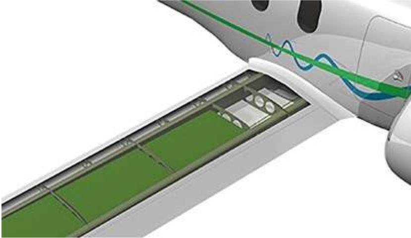
Zunum Aero is proposing to store the batteries for its new electric aircraft design in bays for modular battery packs within the in the wings. (Zunum Aero)
