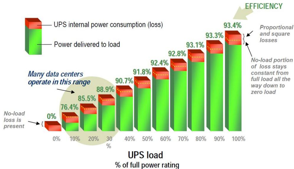
**Figure 2: Breakdown of total UPS input power (Sawyer, 2006)<sup>2</sup>**
