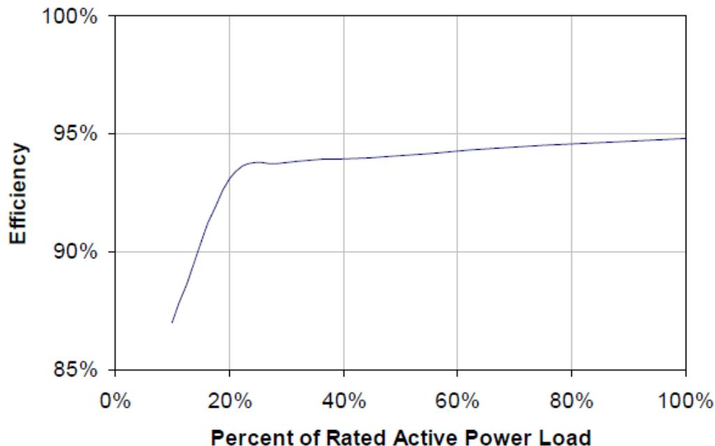
**Figure 1: Typical UPS efficiency curve (PIER, 2008)<sup>1</sup>**
