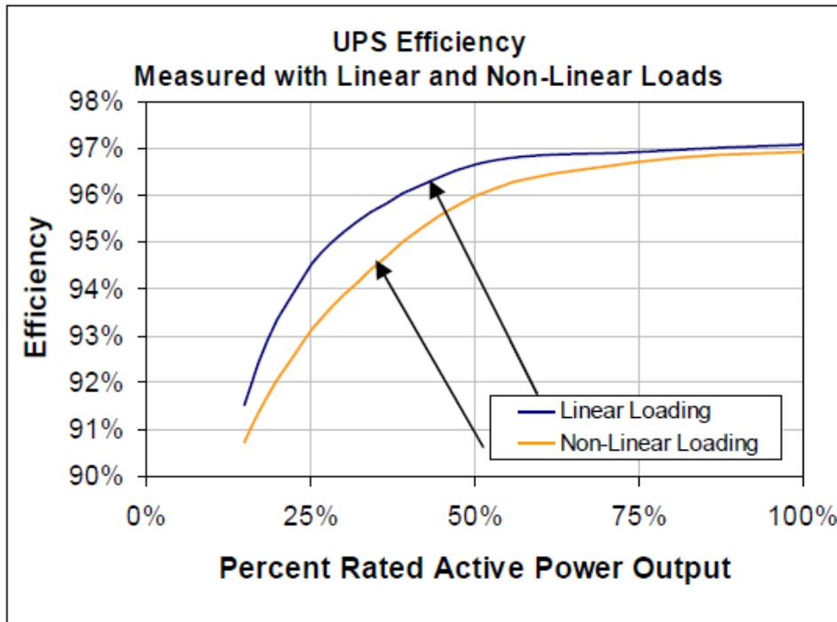
Figure 4: UPS efficiency with linear and non-linear loads (PIER, 2008)<sup>3</sup>
